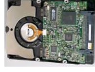
HDD Control Unit
